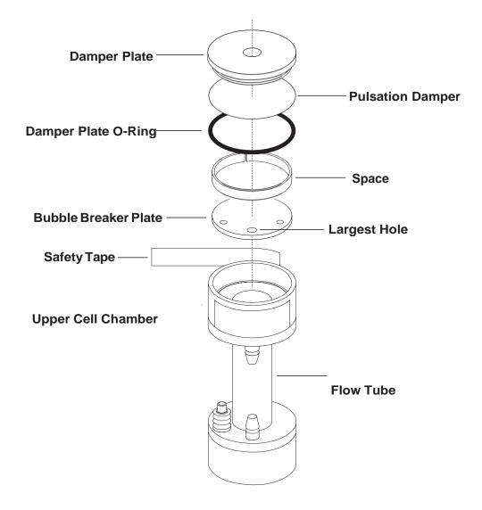
Figure 5.1 Wet Cell Assembly Maintenance
