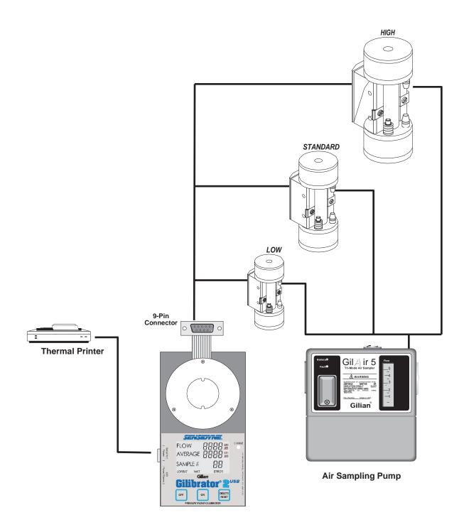
Figure 3.1 Gilibrator 2 System Setup
