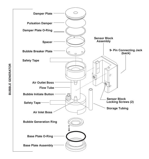
Figure 2.3 Wet Cell Assembly (Exploded View)
