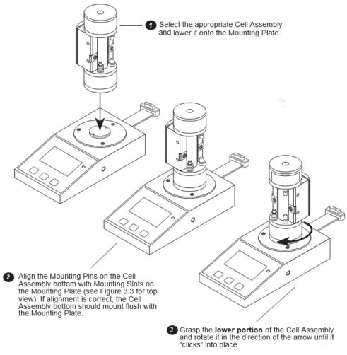
**NOTE**: Always grasp *lower portion* when mounting or removing the Flow Cell.
