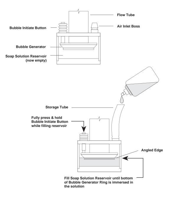
Figure 3.4 Adding Soap Solution (Wet Cell)
